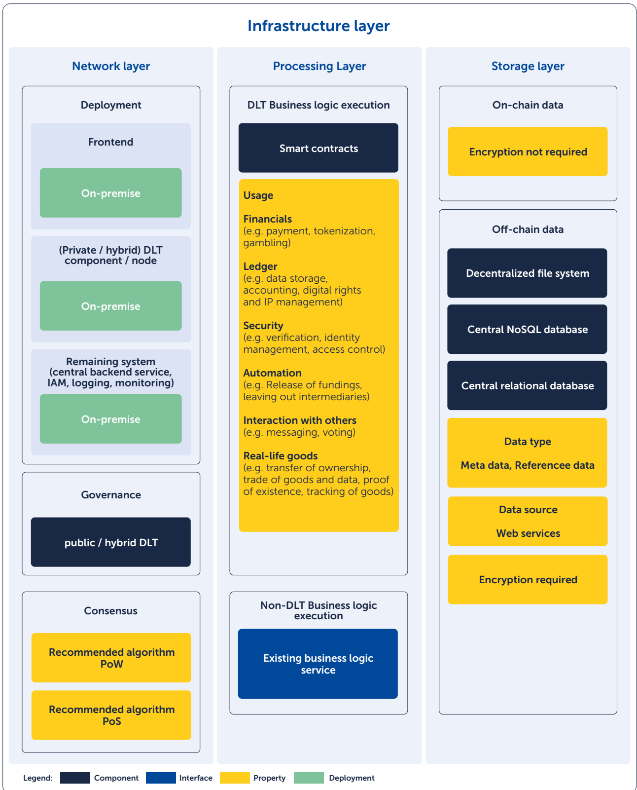
Figure 26: Example DLT-Use-Case-Solver output canvas infrastructure layer
